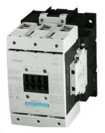
CONTACTOR, 90KW/400V/AC-3 AC(40...60HZ)/DC OPERATION UC 23-26V AUX. CONTACTS 2NO+2NC 3-POLE, SIZE S6E BAR CONNECTIONS CONVENTIONAL OPERATING MECHAN. WITH BOX TERMINAL 3RT19 56-4G TILL 120 MM
